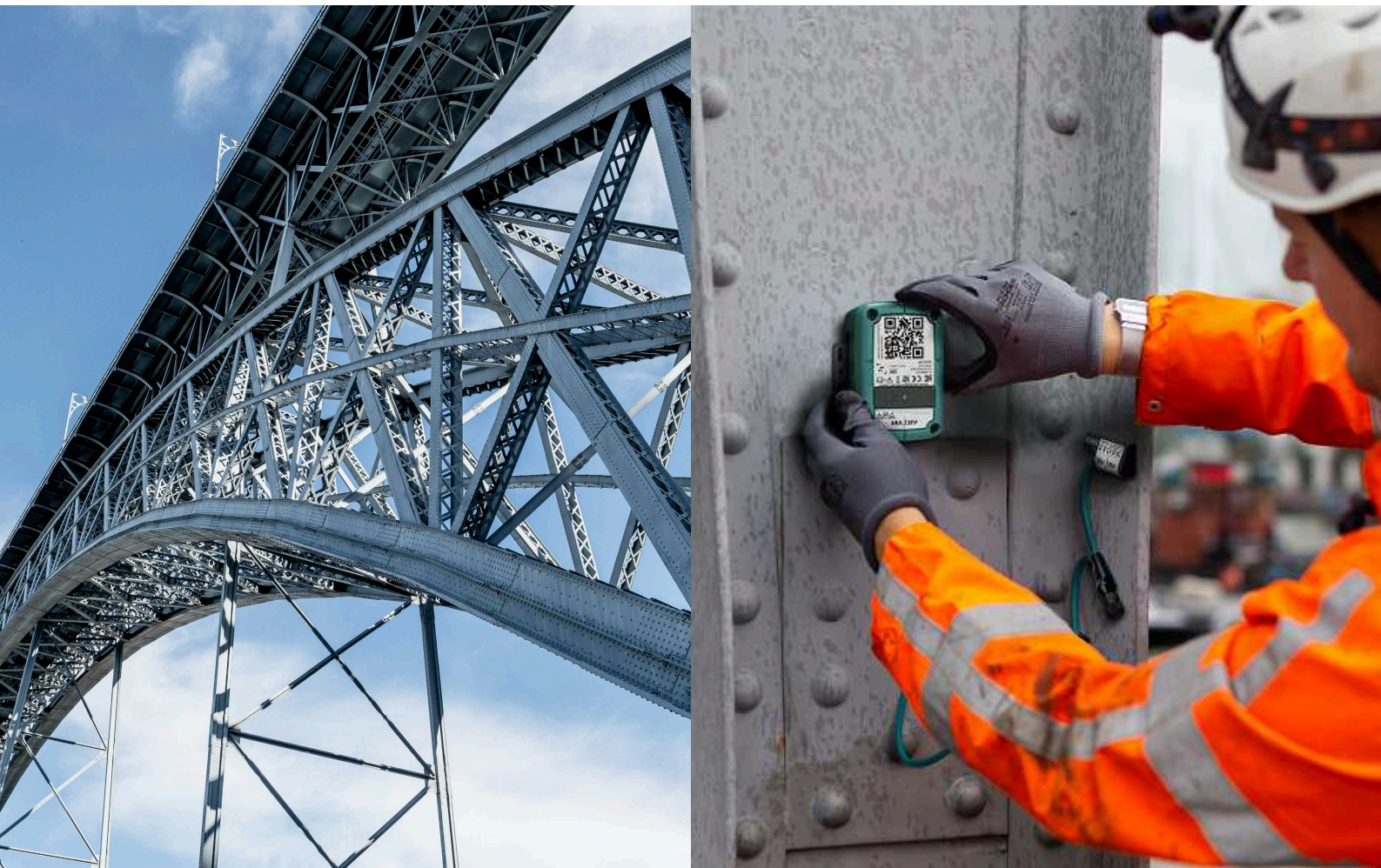
Figure 1 (Left) This image illustrates a steel bridge. (Right) Villari's crack detection sensors are typically installed at critical stress points, to ensure continuous monitoring and proactive maintenance.
