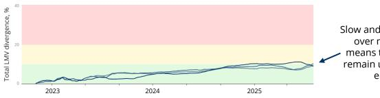
Slow and steady LMV rise over multiple years means the crack might remain unrepaired until end-of-life
